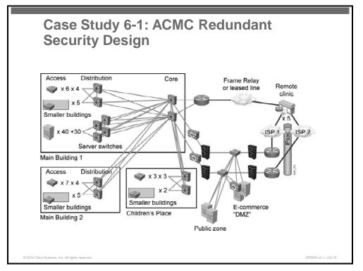
IPS devices were added to this design because an organization investing in this kind of redundancy would probably consider security important enough to want to use IPS devices. Note that an IDS also monitors accesses to the e-commerce servers. Client VPNs can easily be terminated at the firewalls or the IPsec router or routers, to add remote access for doctors or other users.
