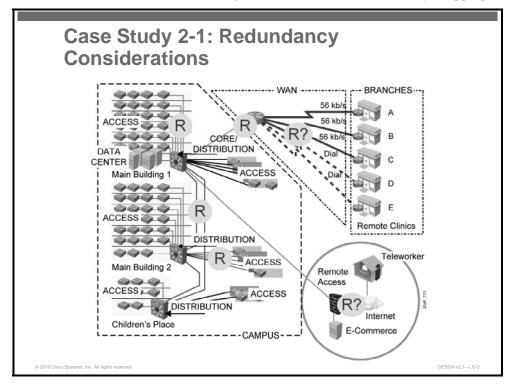
The circled "R" in the diagram indicates where redundancy is appropriate.
