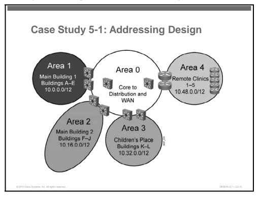
**Step 5** (Optional) Go back and rework the design, treating the small buildings as "floors" of a fourth large campus building and the remote clinics as "floors" of a fifth.
