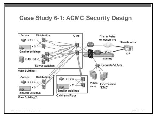
With a suitable PIX Firewall model, you can trunk the VLANs to a switch, with the VLANs separating the public zone and the e-commerce zone or DMZ. The firewall would also secure outbound Internet traffic from ACMC (Internet access for the main campus).
